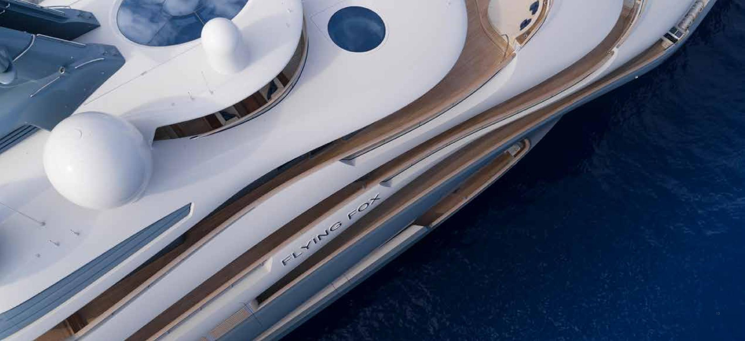
LYING FOX is built with a steel hull and an aluminium superstructure. The shapely curves have been an enormous challenge for the welders. Perhaps even more amazing is her performance: FLYING FOX is capable of 20 knots flat, with a cruising speed of 15 knots.
